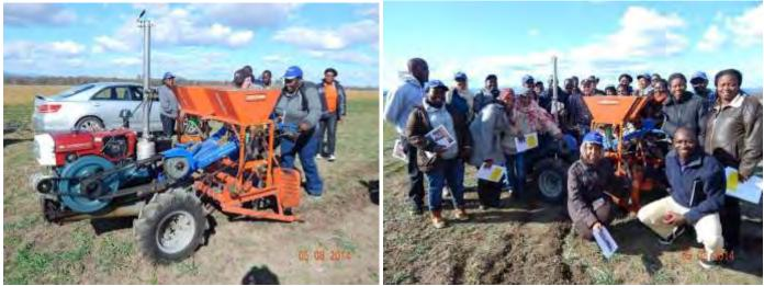
As the ground following tine setup has not yet been completed, the seed drill was set up in a standard two row rigid tine and tool bar arrangement to show the visitors. The various alternative systems of seed metering and alternative soil engaging tools were shown in a nearby static display.
