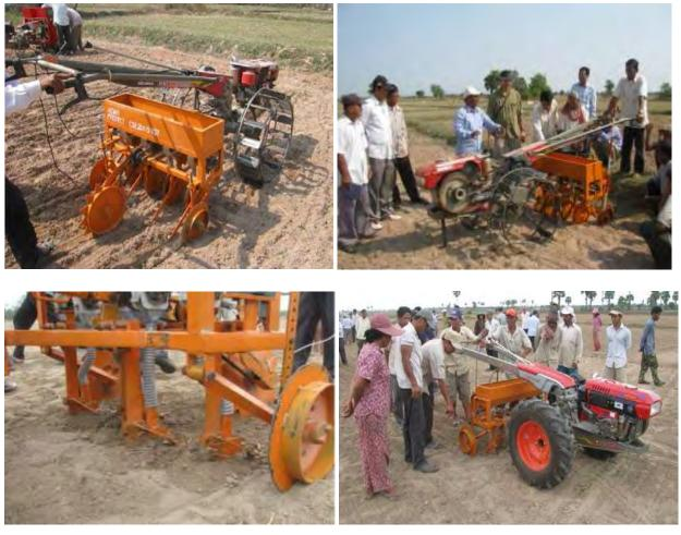
SE-2009-037 project developed Cambodian disc and tine drill prototypes demonstrated in the provinces
