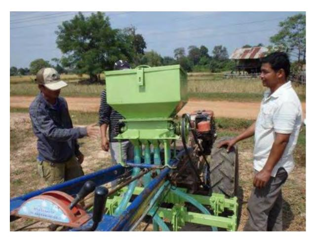
Related to the above unit, Dr Leigh Vial of IRRI has developed a modified form of the Thai direct rice seeder that allows placement of fertiliser in line with the direct seeded rice. This seeder has design features from the original ACIAR-Rogro two wheel tractor seed drill (now the ARC Gongli), as well as the Thai built unit.
