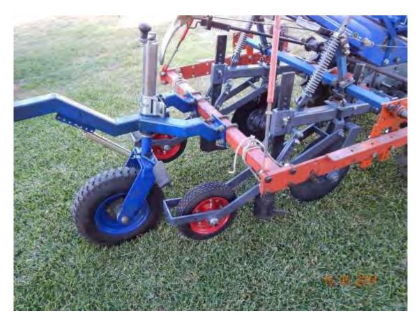
This is a right hand rear view of the complete assembly. The lift system is yet to be completed, along with the seed box frame and seed and fertiliser metering units.
