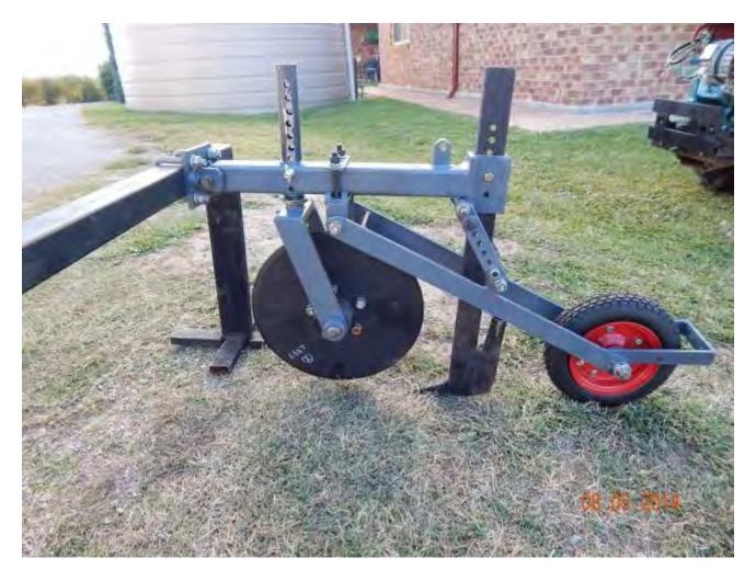
This shows a complete tine unit, complete with the optional cutting coulter. The tine is a standard 50 x 12 hi tensile steel piece, with non-detachable hard faced point. Point rake angle is 30 degrees to minimise draft. The cutting coulter is 356mm (14 inches) in diameter, and swivels. The camber angle of the yoke for the coulter is 20 degrees (with a larger camber angle the coulter has insufficient clearance to the tine).
