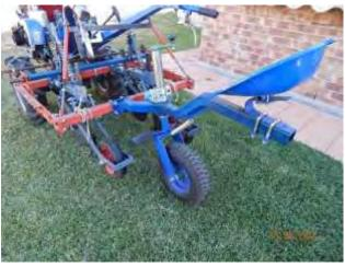
The left hand picture shows the raise-lower system with the pressure/helper spring. The control lever is yet to be constructed. Also a new seed box frame will be built so that is does not hinder any of the mechanisms. Note that the tine assemblies are adjustable for row (line) spacing which is variable from 60-90 cm row width.
