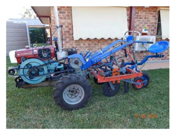
This shows the complete setup with the tines attached to the tool bar. Each assembly must be compact, to fit between the front and rear tool bars, and yet not be obstructed by the handlebars or other parts of the 2WT.
