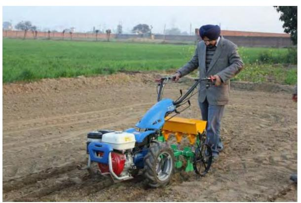
This is a small (around 8HP) petrol operated 2WT with an Indian made rice seed drill attached. Lao research workers are considering this unit as an additional option for direct seeding of rice by small area farmers.
