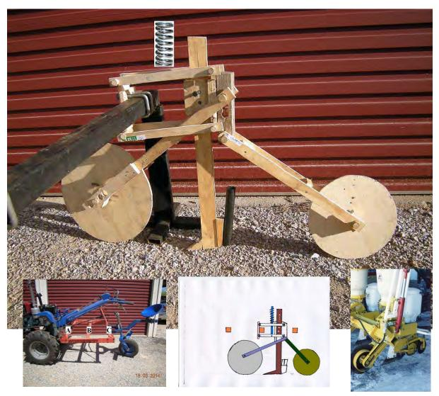
The large picture shows the wooden mock-up of this opener. This design has been derived from a relatively common parallelogram floating tine opener. (Centre insert). A Buffalo tine planter unit (RH insert) is shown as an example. There are many rowcrop planters of this configuration. Early types had the tine only, and most later units now have a cutting coulter as well
