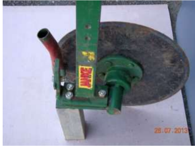
Angled single disc – side view. Note the offset of the frame to the position of the main axle. The angle of offset can be adjusted by loosening the two rear bolts.
