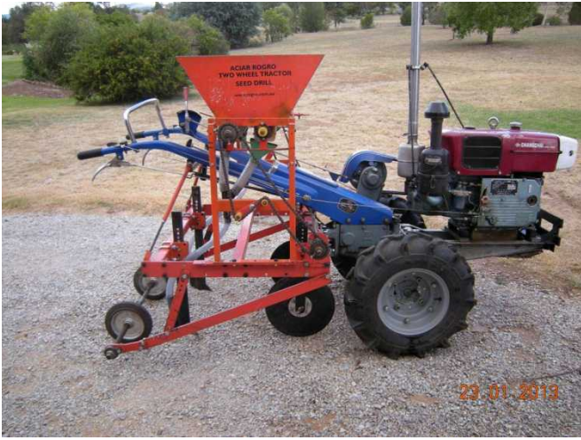
2WT seed drill with disc option fitted to bars 1 & 3 (Note no operator stand fitted)
