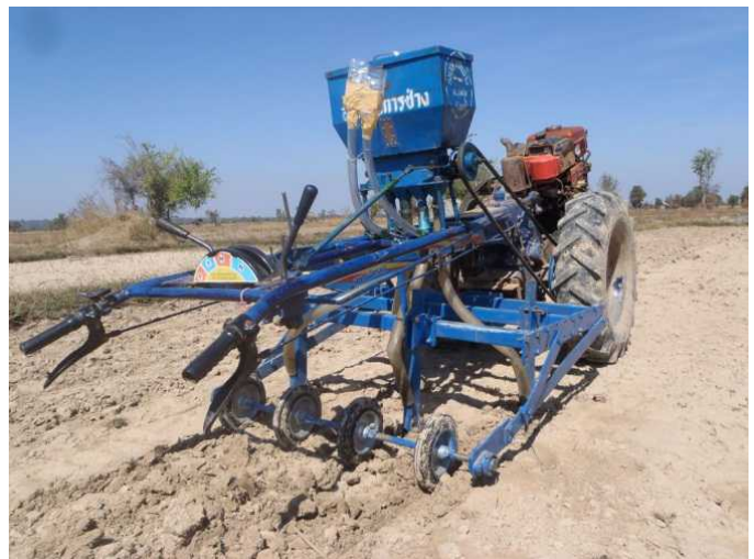
Lao built 2WT seed drill planting dry season rice (zero tillage)
