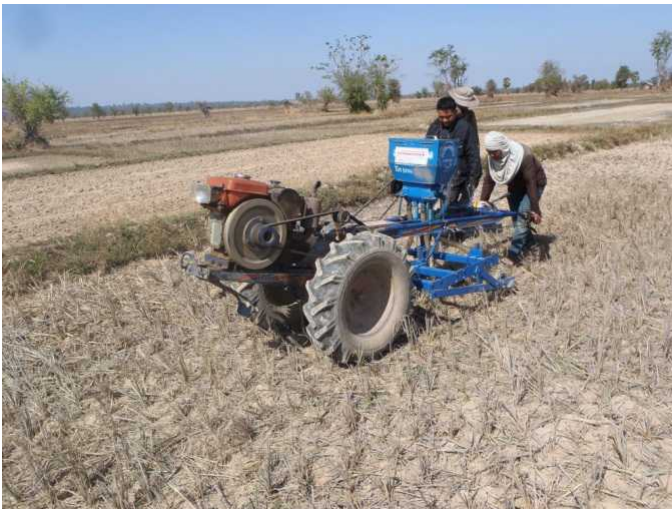
Lao built 2WT seed drill planting dry season rice (zero tillage)
