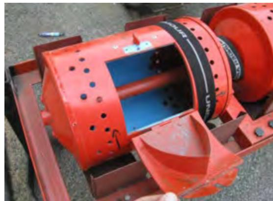
Left: Messrs Chea Sovandina, Prum Cham Roeun and Chuon Sarom of GDA DAEng who developed the 2WT powered drum seeder prototype. Right: Close view of the drum with inner agitator
