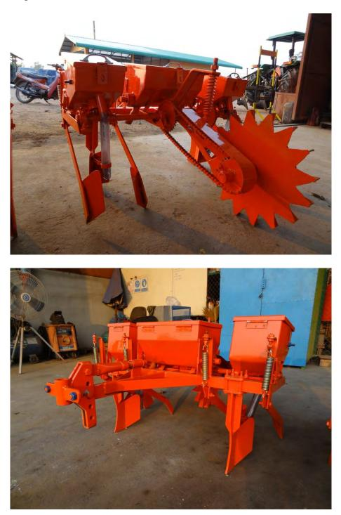
Clive Murray (Syngenta Foundation SE Asia) has supplied me with two pictures of a Thai made 2WT planter. I do not have any detailed information on this planter. However it appears to be fitted with a pair of inclined plate seed metering systems on the seed boxes. The seed covering devices and the drive system is clearly visible.
