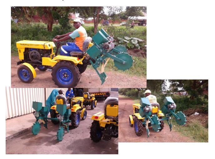
I understand a shipment of small Chinese 4WT has been made into Zimbabwe recently. A two row maize planter, specifically designed for these tractors has been fabricated by a local consortium, comprising the importer and a local farm implement manufacturer. I do not have specific details at this time.
