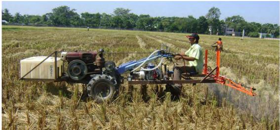
This Bangladeshi made 9 nozzle sprayer is mounted to the 2WT. The centrifugal pump/integral motor unit along with other controls are fitted to a tray under the handlebars, and the Australian made boom is behind the operator.
