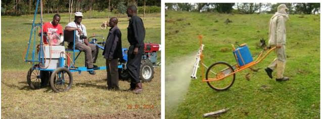
The sprayer on the left was fabricated by Joseph Mutua (KENDAT Kenya) and a wheel barrow model on the same principle is shown on the right. A ground wheel drives the hand pump via a chain and pitman arm.
