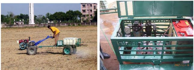
This Bangladeshi one is a trailing 8 nozzle unit. It has a 12V diaphragm pump, 150 litre tank, and is on 800mm track. It is powered by an automotive battery which has to be re-charged every few hours. It has a locally made folding boom.
