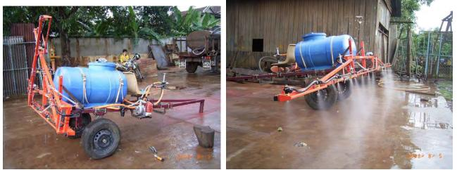
This trailing unit was made in Cambodia in co-operation with CIRAD. It has a centrifugal pump close coupled to a small petrol motor. It has a 10 nozzle Australian made boom, and a locally sourced 300 litre tank.
