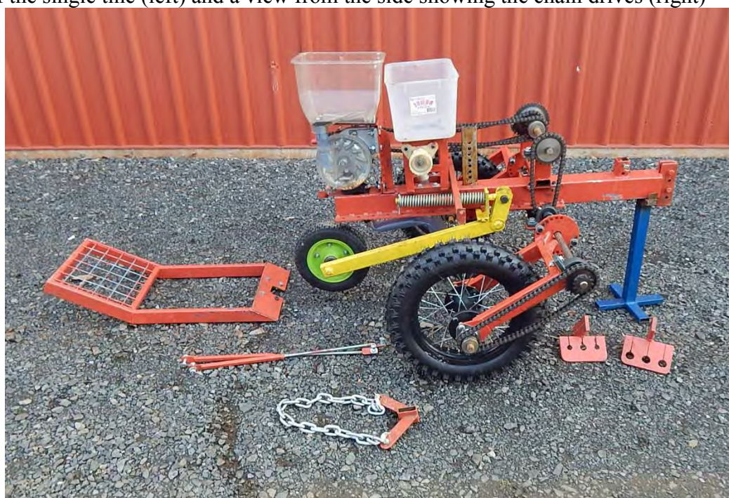
An overall view of the planter showing the press wheel, 12 spoon vertical seed meter, fertiliser mechanism, and the optional operator stand, support struts, covering chain harrow and tractor hitch (2 types available)
