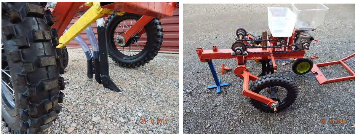
Details of the single tine (left) and a view from the side showing the chain drives (right)
